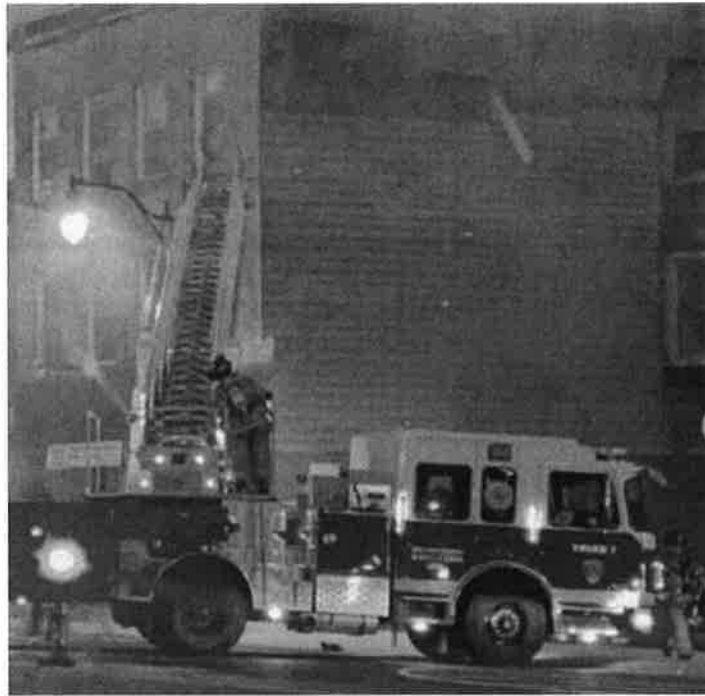
Photos & Drawings 5: Aerial ladder being used for rescue of occupant from third floor window and/or to bring firefighting personnel to the third floor for search and rescue or ventilation operations. Third floor is out of reach for ground ladders
