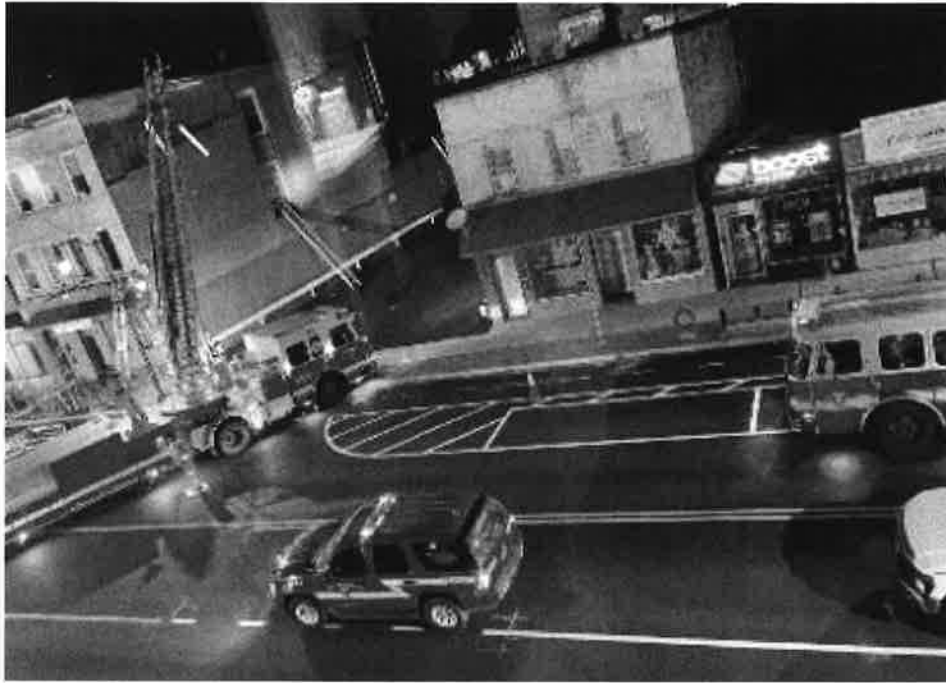
Photos & Drawings 7: Kingston Fire scene in downtown structure fire (1): Fact 28: Fire Incident Street scene of apparatus showing 2 ground ladders placed at windows of a structure fire. Note that the ladder in the front of the building is placed on a roof type structure over the sidewalk rather than to the body of the main structure. This is a dangerous practice because this type of structure is often unstable and prone to collapse.
