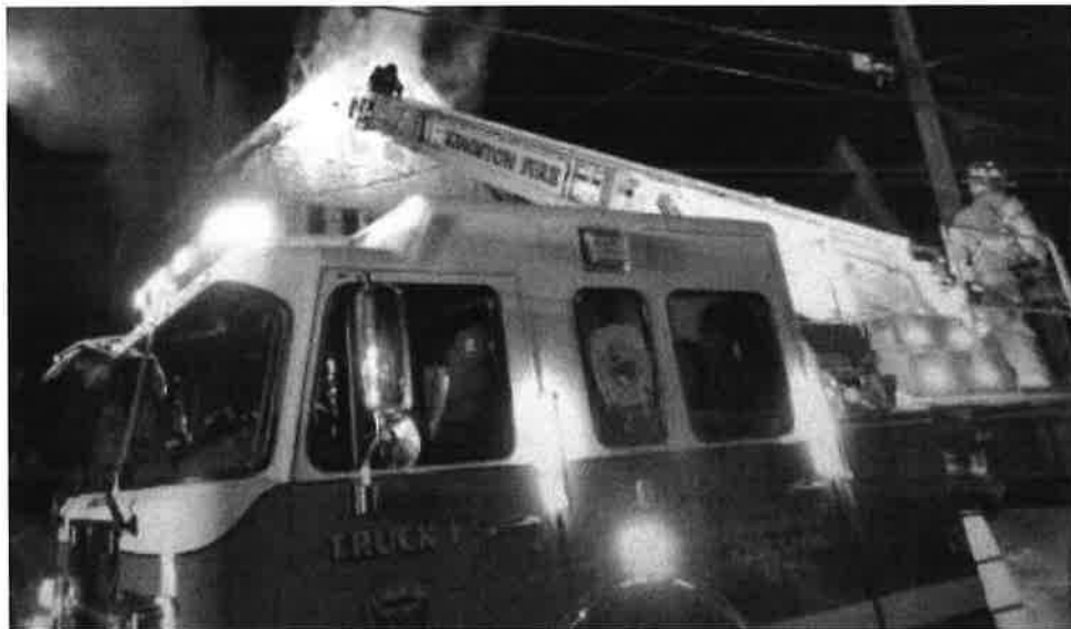
Photos & Drawings 6: Firefighters using the aerial ladder to perform ventilation of an attic window at a house fire. That attic window is out of reach from ground ladders. Note the electric power supply line to the house under the extended aerial ladder.
