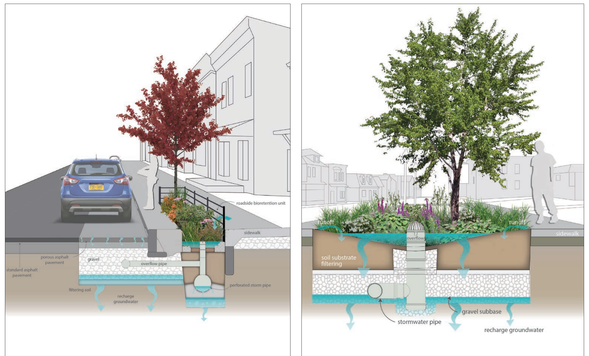
Diagrams of bioretention strategies including porous pavement and rain gardens
