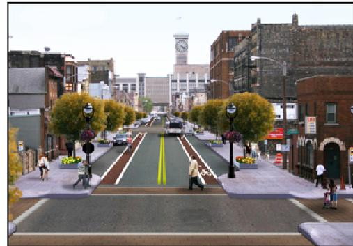
**Above:** Image of complete street in Knoxville, TN with similar dimensions to Broadway in Kingston. The roadway configuration incorporates wide sidewalks, clearly defined crosswalks, designated bike lanes and two travel lanes for motor vehicles.
