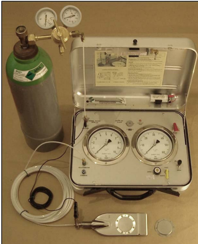
Figure DMT-1. Flat plate dilatometer system (Marchetti, http://www.marchetti-dmt.it/pagespictures/blade&case.htm )
