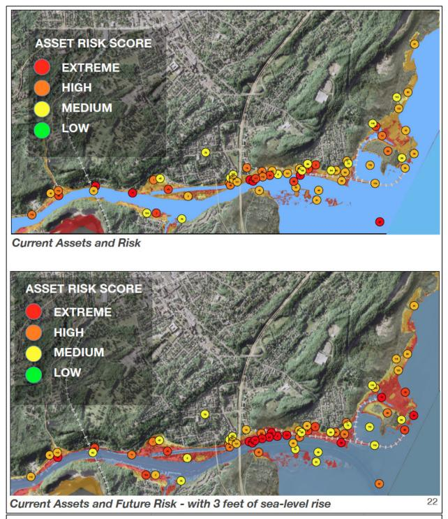
**Source:** Maps from Planning for Rising Waters: Final Report of the City of Kingston Tidal Waterfront Flooding Task Force 2013: showing current assets and risks from flooding under current conditions and future risks with 3 feet of sea-level rise.
